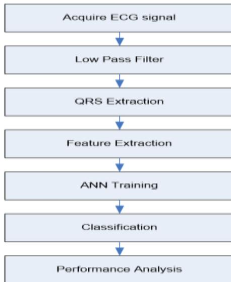
Figure 1: ECG Signal Analysis Framework
