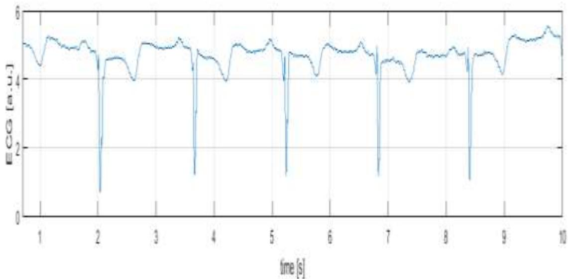
Figure 6: Second-order Butterworth low-pass filtered ECG Signal
