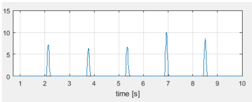
Figure 7: Detected QRS complex
