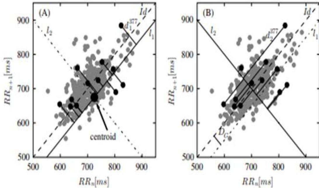
Figure 3: Calculation of the standard Poincare plot descriptors with the use of geometric language. The value of DC, which is the perpendicular distance from the identity line to the centroid (or 11), is exaggerated by a few orders of magnitude for better readability. Id stands for Identity line.
