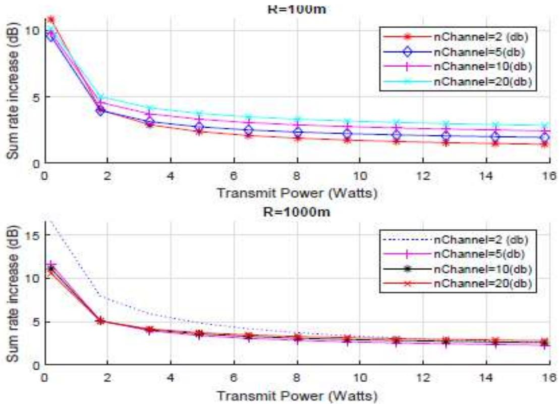
Figure 7: Capacity gain comparison for different number of users at different cell radius.
