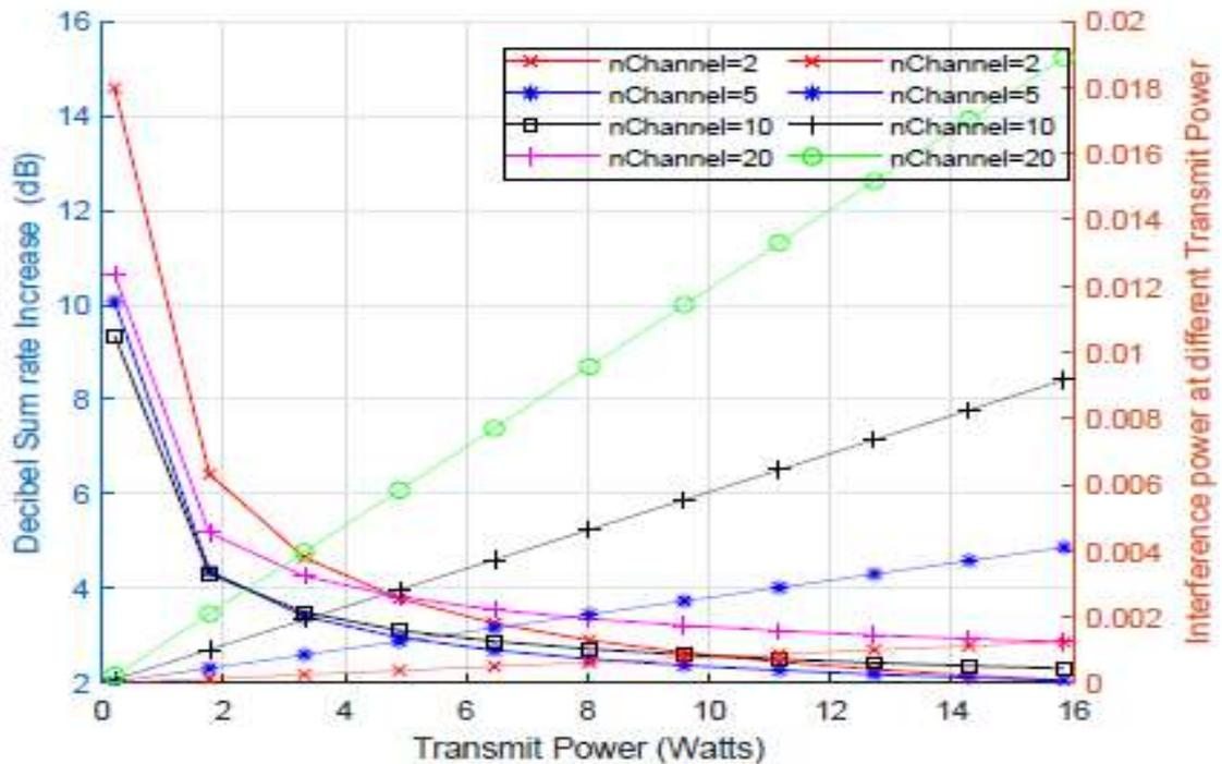
Figure 4. Trade-off between sum rate gain and interference power.
