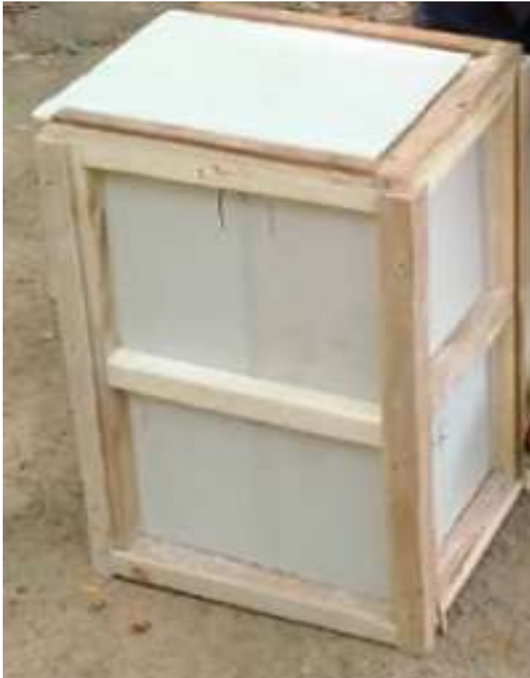
Figure 2: Ceiling materials cubicle used as simulation for house ceilings for house ceilings
